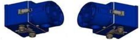
The Double Pass Models use the transmission measurement technique (a folded beam transceiver arrangement) in which a light emitted from the transceiver passes across the stack to a reflector, which then returns the light to the transceiver, where the intensity of the received light is measured. Increased particulate or smoke density in the stack gas attenuates the transmitted light and causes the intensity of the received light to fall which is correlate to the dust concentration in stack.
